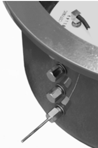
Fig. 10 - Fitting being screwed into the Outlet Port
