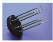
Long pin prod – for testing grain in bulk (requires H-3 Handle)
