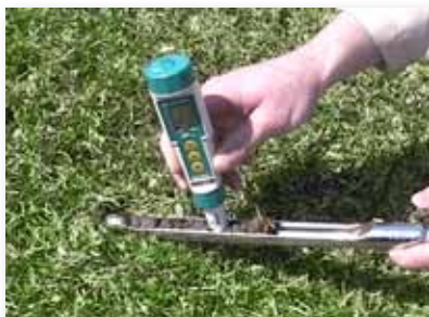
SoilStik shown in use with Item 6510, Model HC Soil Sampler
