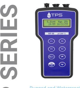
Rugged and Waterproof User Friendly GLP Compliant Automatic Datalogging USB Data Download (optional) Multiple Power Options The WP series is fully waterproof to IP67 and is designed for maximum durability for the harshest conditions. The WP Series is ideal for environmental field testing, laboratory and industrial use.
