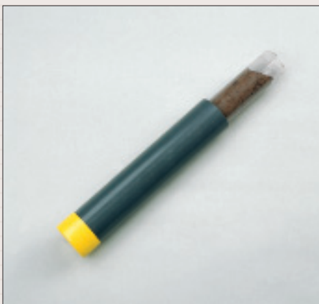
Sample liner container with sample
