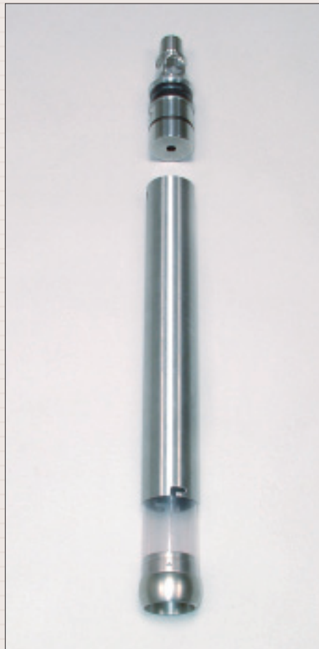
Coring apparatus, tube, cutting head
