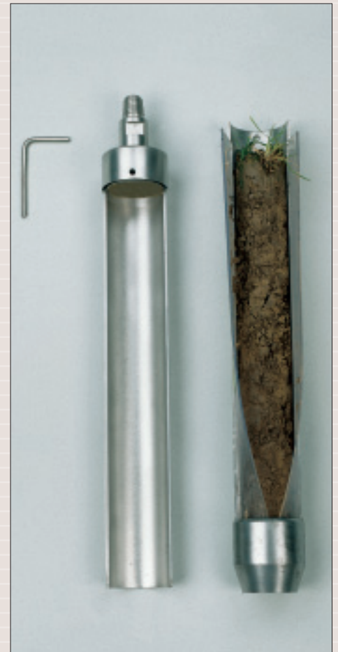
Split tube sampler with sample in liner
