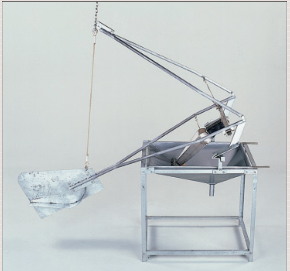
Bed load transport meter, Arnhem type
