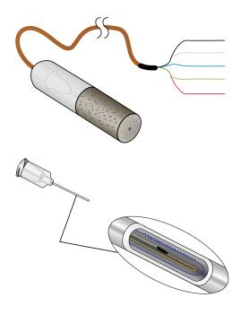
A 229 Heat Dissipation Matric Water Potential Sensor is shown at the top. The hypodermic assembly (without epoxy and ceramic) is shown just below. Cutaway view shows longitudinal section of the needle with heater and thermocouple junction.
