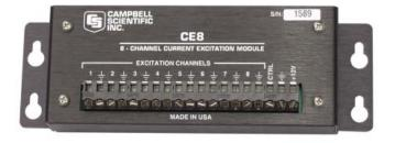
The CE8 can source current for eight 229 sensors directly. The outputs of the CE8 can be connected to as many as eight multiplexers, greatly expanding system capacity.
