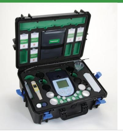
Packed with robust soil testing hardware using simplified versions of laboratory soil testing methods, the SKW 400 includes:
