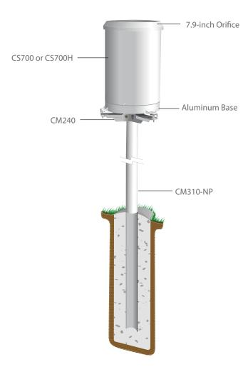
The CS700 and CS700H have a powder-coated aluminum base. The above rain gage is mounted onto a CM310 pole via the CM240 mount. The CM310 pole is embedded directly in a concrete pad (-NP no pedestal base option).
