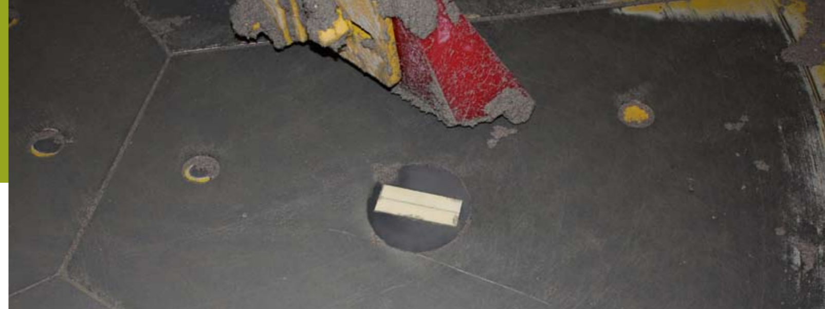
SONO-MIX moisture probe installed into a mixing pan bottom.
