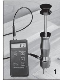
Lignomat's pinless meters for wood, concrete and other building materials are available for a measuring depth of 3/4" and/or 1/4" (20 or 7mm). All pinless meters have built-in corrections for different wood species (2).
