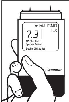
**Check/Change Settings:** Wait until meter turns itself off. Click on-off switch between pins twice. Yellow numbers indicate settings 1-40 for wood and settings 0 and 41 for building materials. To change setting, click on-off switch again or hold switch down to start count. Change Mode is only accessible when meter is off.
