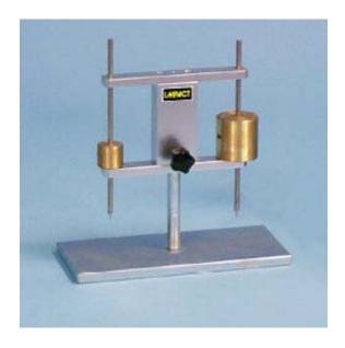
Used to determine the setting time of cement.
