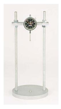
The apparatus consists of a steel frame with a dial gauge mounted on an adjustable height cross-bar.
