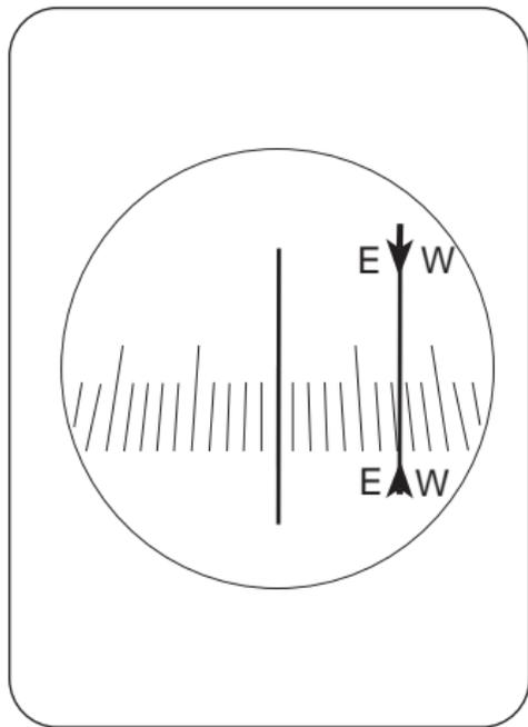
**ATTENTION!** When using the maneuverable sighting line, always take the reading at the same place of the scale line, for instance, at the end of the scale line. Please note that the difference on the scale between the fixed and maneuverable sighting lines is about half of the adjusted declination correction. This is due to the optical structure of the compass.
