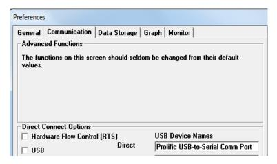
Fig. 3: Hardware Flow Control Option (Specware 9)
