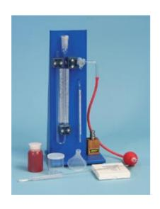
to EN 196-6, COMPARABLE TO, ASTM C204, AASHTO T153, BS 4359:2, UNI 7374, NF P15-442 -UNE 80-106
