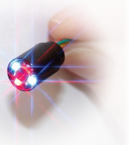
Optical DO sensor LED's flash during measurement.
