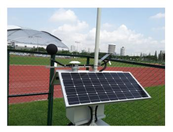
• Measurement of black globe temperature in outdoor applications finds its most typical application in the definition of heat stress in public places, in order to warn about potentially dangerous situations for health or for research purposes.
