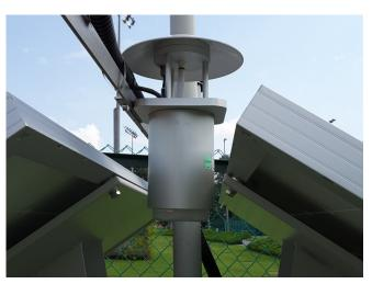
Outdoor measurement of the wet temperature finds its most typical application in the calculation of the WBGT index (ISO 7243) when continuous or outdoor monitoring is required. In these cases, small sensors with little water capacity and inadequate solar shields are not suitable. The DMA121A and DMA122 sensors are the "meteorological" solution for this measurement.
