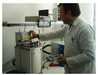
► LSI LASTEM is an ISO17025 accreditated laboratory for air temperature measurements. All sensors manufactured are tested inside our laboratory. LSI LASTEM provides Test report for any sensor supplied and on request, ISO17025 or ISO9001 calibration certificates (see Accessories list).
