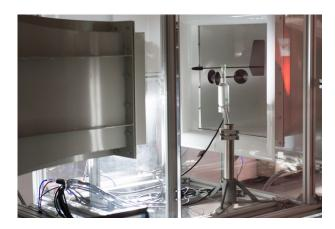
▶ LSI LASTEM is an ISO17025 accreditated laboratory for air speed measurements. All sensors manufactured are tested inside this laboratory. LSI LASTEM provides Test report for any sensor supplied and on request, ISO17025 or ISO9001 calibration certificates (see Accessories list).
